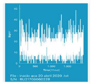
Fig. 3 – Monitoring of 2000-hour series from Radon Eye RD200 in ACA tower using (Bq/m<sup>3</sup>) unit from January 27 to April 20 of 2020
