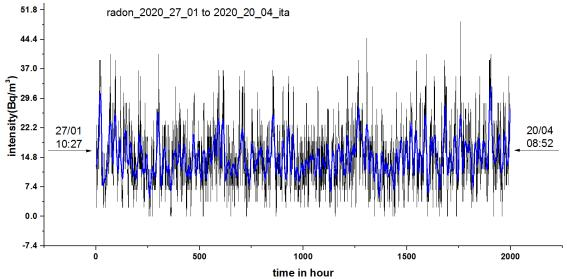
Fig.5 - Monitoring of radon gas from January 27 to April 20, 2020 in ITA. The blue curves corresponding smoothed values in one day
