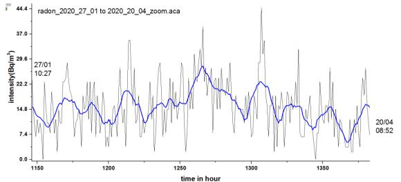
Fig.6 - Increased verification of the interval between measurements from 1000 to 1500 hours seen in figure 4. The variation of radon gas is observed every hour and every day
