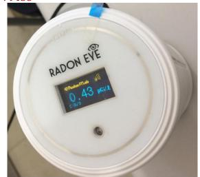
Fig 2 – Top view of RD200 Radon Eye ionization chamber used for monitoring radon gas [8]
